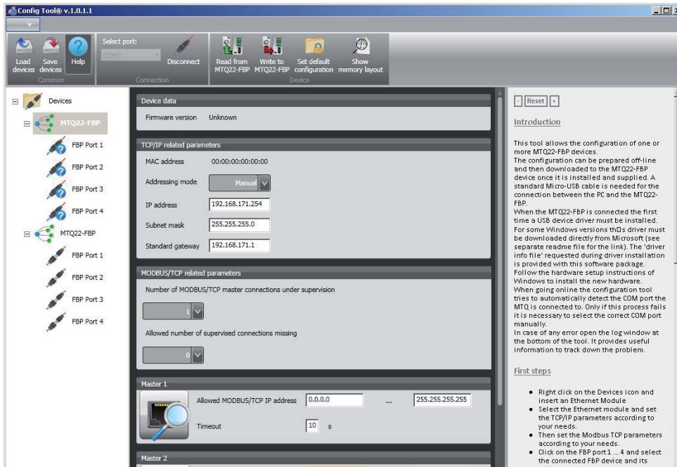
Figure 12: The configuration tool allows to set the parameters in an easy way. Several MTQ22-FBP devices can be created in the device tree (left). The final configuration can be saved to disk and downloaded into the devices using a standard USB cable.
