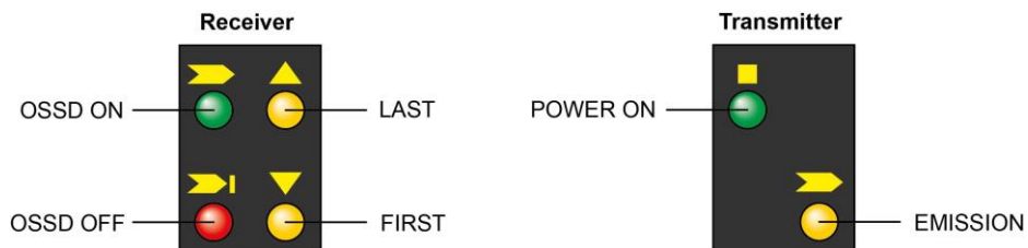
Figure 24 – Displays on transmitter and receiver
