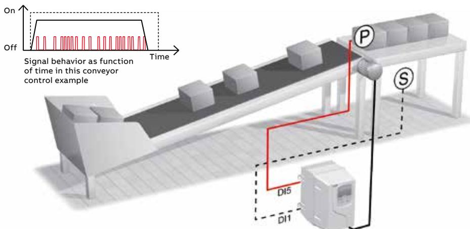
Parameter 1907 COUNTER RESET is set to DI1 (INV) [-1]. When digital input 1 is low, the counter is reset to a value determined by parameter 1908 COUNTER RES VAL.
