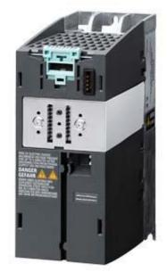
SIPLUS SINAMICS G120 PM 240-2 FSA-1.5kW -20...+50°C with conformal coating based on 6SL3210-1PE14-3UL1 . unfiltered with integrated braking chopper 380-480 V 3 AC +10/-10% 47-63 Hz Power high overload: 1.1 kW at 200% 3s, 150% 57s, 100% 240S Power low overload: 1, 5kW 196x 73x 165 (HxWxD), FSA Degree of protection IP20 without Control Unit and operator panel Released as of firmware version V4.6
