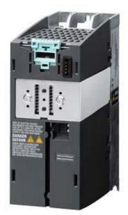
SIPLUS G120 PM 240-2 FSA-3kW -20...+50°C with conformal coating based on 6SL3210-1PE18-0UL1 . unfiltered with integrated braking chopper 380-480 V 3 AC +10/-10% 47-63 Hz Power high overload: 2.2kW at 200% 3s, 150% 57s, 100% 240S Power low overload: 3kW at 150% 3s, 110% 57s, 100% 240S 196x 73x 165 (HxWxD), FSA Degree of protection IP20 without Control Unit and operator panel Released as of firmware version V4.6
