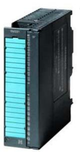
SIPLUS S7-300 SM 331 8AI 40-pole with conformal coating based on 6ES7331-7PF11-0AB0. Analog input isolated, 8 AI thermocouples Type B, E, J, K, L, N, R, S, T TXK/TXK (L) according to GOST 16 bit, 50ms, 1x 40-pole
