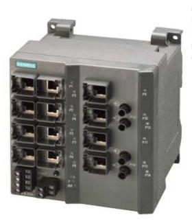
SIPLUS NET SCALANCE X212-2 for medial exposure with conformal coating based on 6GK5212-2BB00-2AA3 . Managed IE switch, 12x 10/100Mbit/s RJ45 ports, 2x 100 Mbit/s multimode BFOC, LED diagnostics, error signaling contact with set button, Redundant power supply, PROFINET IO device, network management, integr. redundancy manager, incl. electron. Manual on CD-ROM, C-plug optional
