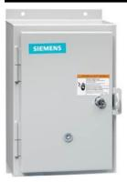
Industrial enclosure kit with hinged door NEMA Type 3/3R/12 Dust tight and drip proof for indoor use Weatherproof for outdoor use Used for field assembly of non-combination type control products.
