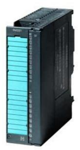
SIPLUS S7-300 SM 331 8AI with conformal coating based on 6ES7331-7PF01-0AB0 . Analog input isolated, 2/3/4-wire, 8 Al, Resistor, Pt100/200/1000 NI100/120/200/500/1000, CU10, characteristics according to GOST 16 (internal 24) bit, 50ms, 1x 40-
