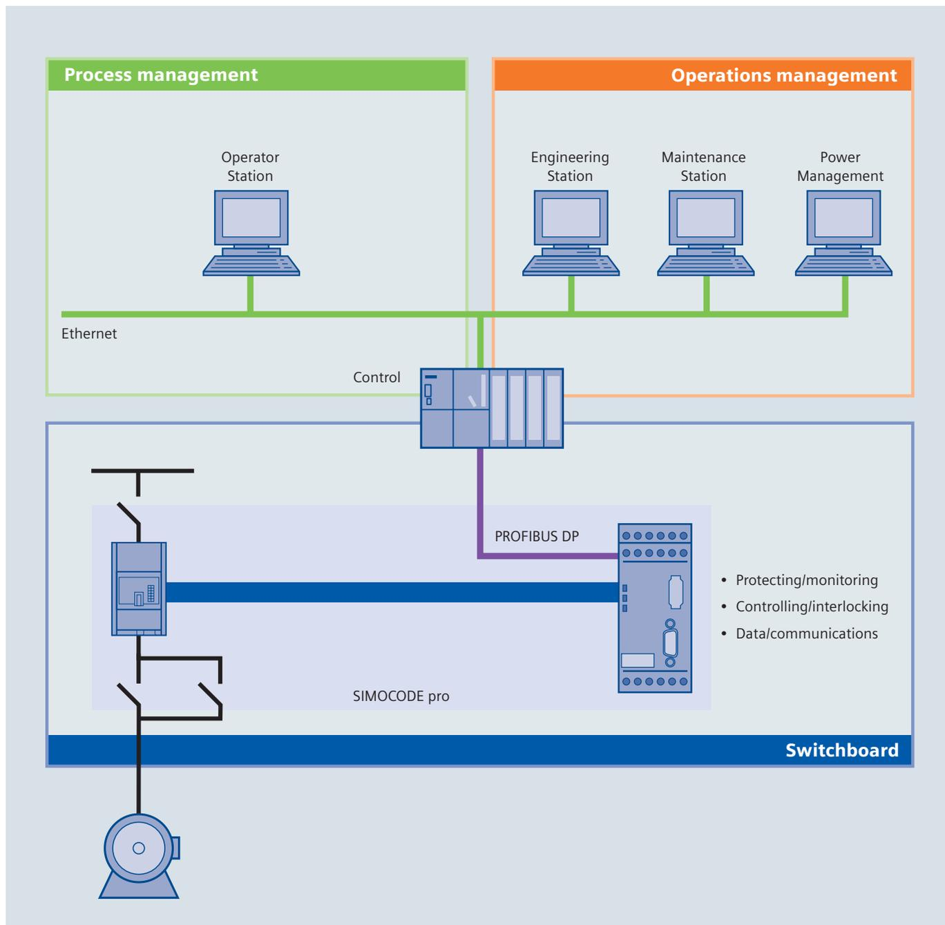
SIMOCODE pro combines all of the functions required for your motor feeder and connects this to higher-level systems via PROFIBUS DP.
