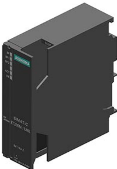
SIPLUS ET 200M IM 153-2 (\*BA02) -40...+70°C start up temperature:-25°C with conformal coating based on 6ES7153-2BA10-0XB0 . Connection ET 200M IM 153-2 High Feature for max. 12 S7-300 modules with redundancy capability, Time stamp. suitable for isochronous mode New features: up to 12 modules can be used Slave Initiative for Drive ES and Switch ES Expanded quantity structure for HART auxiliary variables Operation of the 64-channel modules 32 signals/slot
