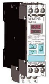
Digital monitoring relay Current monitoring, 22.5 mm from 2-500 mA AC/DC 0vershoot and undershoot 24 to 240 V AC/DC 50 to 60 Hz DC and AC ON delay and noise pulses delay 0.1 to 20 s Hysteresis 0.1 to 250 mA 1 change-over contact with or without fault buffer screw terminal Successor product for 3UG3521-1AL20, 3UG3521-1AG20 and 3UG3521-1AC48-0AA1
