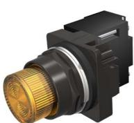
30mm BlackMax, Epoxy Coated Corrosion Resistant Complete Metal Unit Illuminated Indicator Light Transformer type, 240V AC LED Lamp, BA9s Plastic Lens, Amber UL Listed, CSA Certified NEMA 1,3,3R,4,4X,12,13 & Automotive Standards
