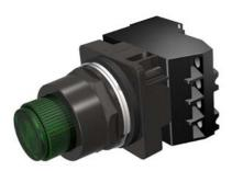
30mm BlackMax, Epoxy Coated Corrosion Resistant Complete Metal Unit PTT / Illuminated Pushbutton Full Voltage, 120V AC/DC Incandescent Lamp Extended Button Plastic Lens, Green 2 Position Momentary with 1 N.O. - 1 N.C. Heavy Duty Contacts, A600/P600 UL Listed, CSA Certified NEMA 1,3,3R,4,4X,12,13 & Automotive Standards
