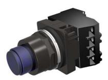
30mm BlackMax, Epoxy Coated Corrosion Resistant Complete Metal Unit PTT / Illuminated Pushbutton Transformer type, 120V AC LED Lamp Extended Button Plastic Lens, Blue 2 Position Momentary with 1 N.O. - 1 N.C. Heavy Duty Contacts, A600/P600 UL Listed, CSA Certified NEMA 1,3,3R,4,4X,12,13 & Automotive Standards
