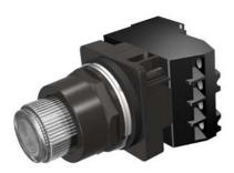
30mm BlackMax, Epoxy Coated Corrosion Resistant Complete Metal Unit PTT / Illuminated Pushbutton Transformer type, 120V AC Incandescent Lamp Extended Button Plastic Lens, Clear 2 Position Momentary with 1 N.O. - 1 N.C. Heavy Duty Contacts, A600/P600 UL Listed, CSA Certified NEMA 1,3,3R,4,4X,12,13 & Automotive Standards
