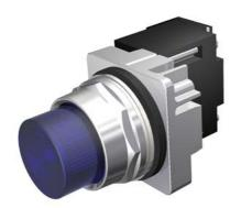
30mm Command/52, Chrome Finish Heavy Duty,Watertight/Oiltight Complete Metal Unit Illuminated Indicator Light Full Voltage type, 24V AC/DC LED Lamp, BA9s Plastic Lens, Blue UL Listed, CSA Certified NEMA 1,3,3R,4,4X,12,13 & Automotive Standards
