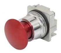
30mm Command/52, Chrome Finish Heavy Duty, Watertight/Oiltight Metal Operator, Round Push-Pull Operator Non-Illuminated Mushroom Head Cap Small 1.73" (44 mm) Metal, Anodized Red 3 Position Momentary UL Listed, CSA Certified NEMA 1,3,3R,4,4X,12,13 & Automotive Standards
