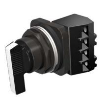
Selector switch, metal, NEMA 4X Spring return from right Long lever, A Cam 1NO-1NC left, right 2 position Complete device white insert Non-Illuminated UL file E22655 in Vol. 6 (7) Sec. 13 (2)
