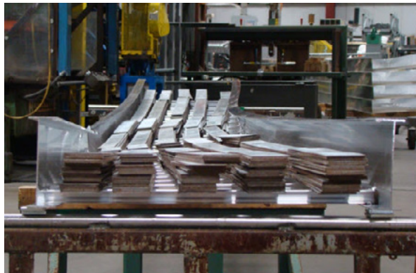
NEMA load test - Worse cast load scenario - Single span with weight applied until physical failure
