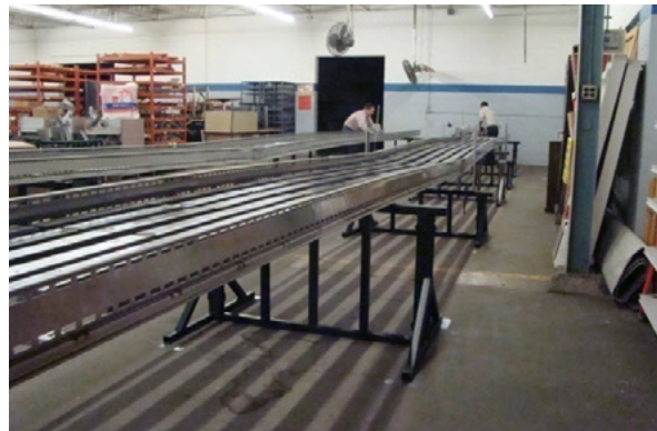
IEC load test - Typical installation scenario Continuous span with weight applied until deflection reaches 1/100 of span length
