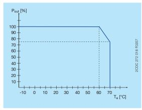
Characteristic curve of temperature at  $\boldsymbol{U}_{\text{out}}$
