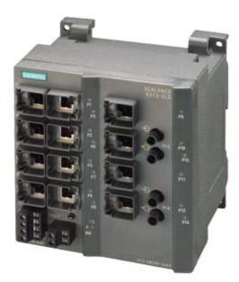
SCALANCE X212-2LD, managed IE switch, 12x 10/100 Mbit/s RJ45 ports, 2x 100 Mbit/s single-mode BFOC, LED diagnostics, error-signaling contact with set button, redundant power supply, PROFINET IO device, network management, Redundancy Manager integrated, incl. electron. manual on CD-ROM, C-plug optional
