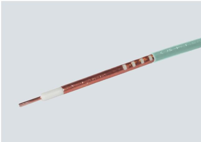
The RCoax cables are radiating cables that function as special antennas for the SCALANCE W Access Points in environments with complex radio coverage. Its design means that a defined, cone-shaped radio field is generated along the RCoax cable. The radiating cables are therefore perfectly suitable for use in all types of applications with track-bound vehicles.
