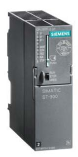
SIMATIC S7-300, CPU 317F-2DP, Central processing unit with 1.5 MB work memory, 1st interface MPI/DP 12 Mbit/s, 2nd interface DP master/slave Micro Memory Card required Can be used with software package S7 Distributed Safety V5.2 SP1 or higher
