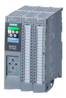
\*\*\* Spare part \*\*\* SIMATIC S7-1500 Compact CPU CPU 1511C-1 PN, central processing unit with work memory 175 KB for program and 1 MB for data, 16 digital inputs, 16 digital outputs, 5 analog inputs, 2 analog outputs, 6 high-speed counters, 4 high-speed counters for PTO/PWM/frequency output 1st interface: PROFINET IRT with 2-port switch, 60 ns bit performance, incl. push-in front connector, SIMATIC Memory Card required
