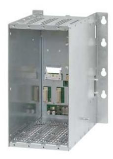
SIPLUS HCS4200 RACK4200 for holding up to 4 power output modules (POM) POM4220. The POMs are contacted via direct connectors on a bus PCB which of the rear of the rack connected. Communication to the higher- level controller takes place via the central interface module (CIM), which is attached on the left side of the rack
