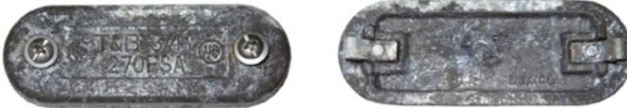
The T&B Fittings sand cast covers still shows no signs of pitting or red rust either inside or out. Only salt deposits.
