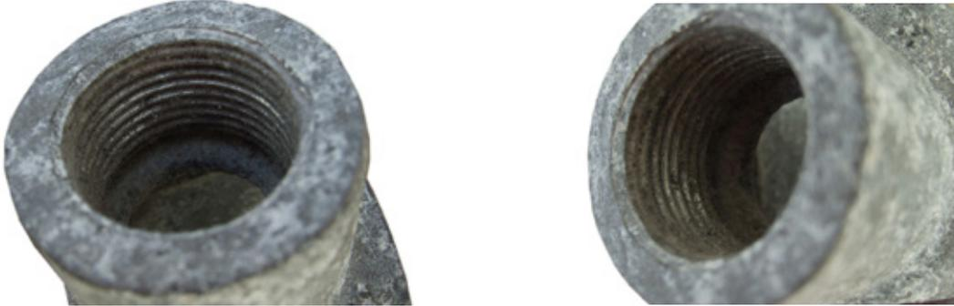
The T&B Fittings conduit bodies display clean threads with only salt deposits.
