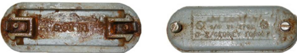
Competitor 2 covers have also been heavily affected by red rust both in and out, despite an additional paint layer.
