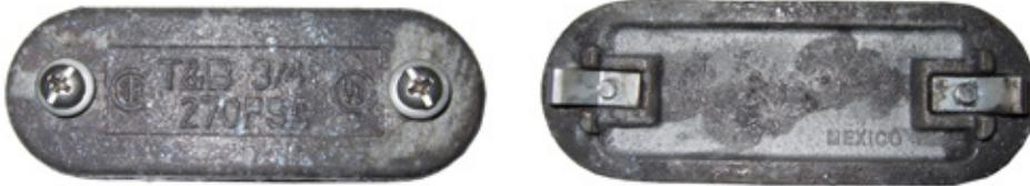
The T&B Fittings sand cast cover shows no signs of pitting or red rust either inside or out.
