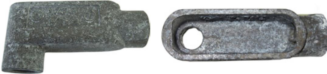
The T&B Fittings conduit bodies are free of any pitting inside and out—only salt deposits.
