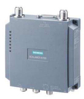
IWLAN client, SCALANCE W738-1 M12, 1 radio, 2 N-CON antenna port, iFeatures support via key plug, IEEE 802.11a/b/g/h/n, 2.4/5 GHz, gross data rate 300 Mbit/s, 2x M12 max. 100 Mbit/s, PoE integrated 2-port switch, redundant 24 V DC,M12 A-coded IP65, - 20... 60 °C, plug slot WPA2/802.11i/e, observe national approvals! CERT ID: MSN65-W1-M12-E2 Scope of delivery: Manuals on CD-ROM, English/German; M12 sealing caps, for operation in the USA
