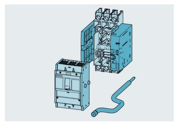
As with plug-in technology, with draw-out technology, the 3VA UL molded case circuit breaker is equipped with plug-in contacts for the main circuits. In addition, side walls including guide and retaining studs are screwed onto the side of the molded case circuit breakers.
