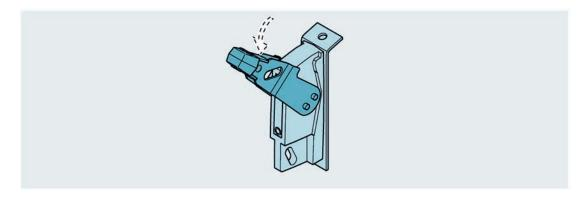
The molded case circuit breaker remains in the tripped state until the manual operator is reset:
