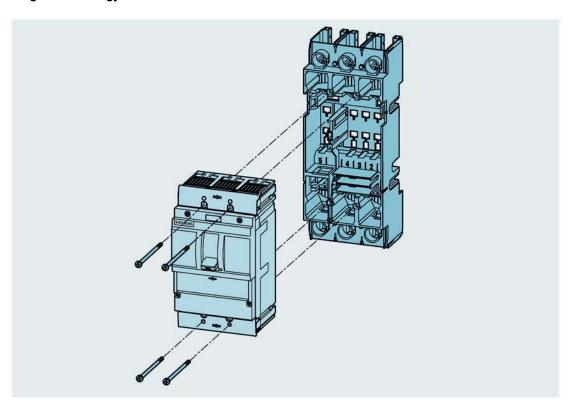
Plug-in technology is the less expensive and more space-saving of the two solutions. Here, the molded case circuit breaker in inserted into the corresponding socket and equipped with plug-in contacts that establish a force- and form-fitted connection with the mating contacts in the plug-in socket – the tulip contacts. In this case, the device is plugged in and withdrawn manually.
