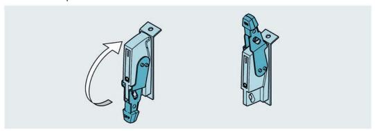
To open the 3VA UL molded case circuit breaker:
