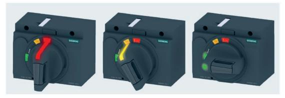
You can retrofit an active illumination kit to manual rotary operators. The illuminated indicator in the rotary handle signals the relevant breaker position in the colors red, yellow and green. This provides clear visualization of the breaker position on-site in conditions of poor visibility.
