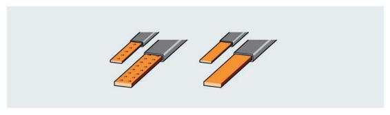
Rigid busbars are made of copper or aluminum. Pre-punched aluminum busbars, some of which are threaded, are often used.
