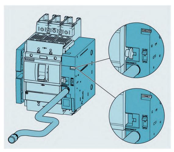
In the case of draw-out technology, the 3VA UL molded case circuit breaker is mounted on the side walls and can be moved into three defined positions by turning the crank handle. The current breaker position is indicated by the breaker status indicator.
