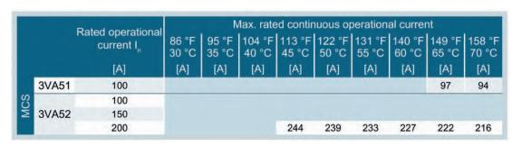
No derating up to the rated operational current In of the molded case circuit breaker
