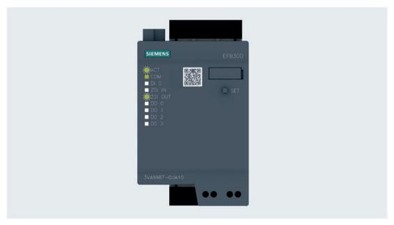
5. In order to select the next output, press the <SET> button briefly ①. The LED of the next output starts to flash ②, the output is selected.
