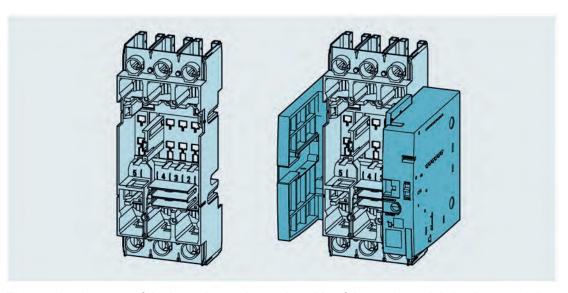
The termination area of the incoming and outgoing side of the socket unit is implemented the same as the associated 3VA UL molded case circuit breakers. The major benefit of this is that all terminal and connection variants including terminal covers of the 3VA UL molded case circuit breaker can be used with the corresponding plug-in or draw-out unit without limitation.
