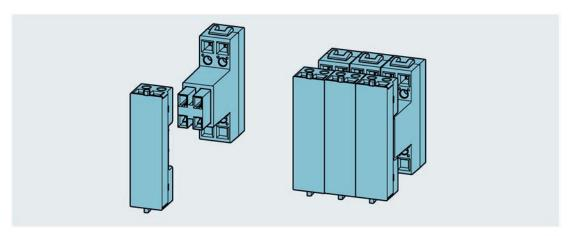
The part of the auxiliary circuit connectors on the circuit breaker side is mounted on the underside of the molded case circuit breaker using the cable cage and is electrically connected to the internal accessories. Appropriate openings and cable ducts are provided in the molded case circuit breaker for routing stranded wires. The plug-in socket half of the auxiliary circuit connector is inserted in the socket and electrically connected to the customer's installation.
