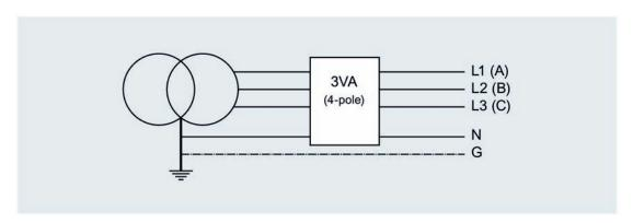
Trip unit variants, 4-pole 3VA6 molded case circuit breaker:
