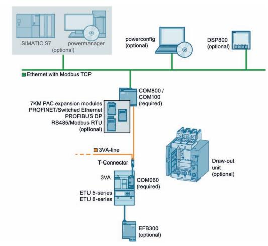
The central components of communication-capable 3VA UL molded case circuit breakers are the ETUs 5-series and 8-series.
