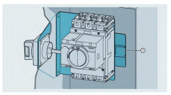
If there is insufficient space available on the mounting plate to install terminals, a terminal plate ① can be bolted to the panel.
