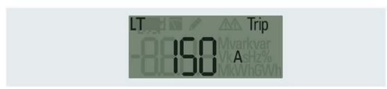
This screen can be identified by the word "Trip" which is displayed in the top, right-hand corner. The displayed current value shows the current at the moment of tripping.
