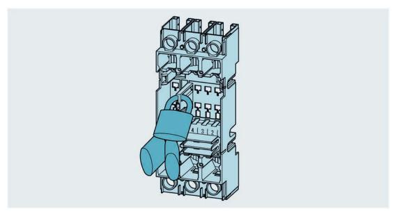
The socket unit can be locked with padlocks to prevent unauthorized insertion of a molded case circuit breaker during service calls and inspections. Using these locks to prevent insertion and operation of a molded case circuit breaker helps to protect personnel and the installation itself. The socket unit of the plug-in socket is equipped with three openings for padlocks.
