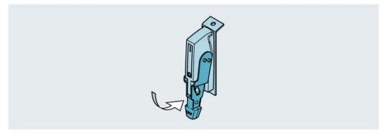
3. Turn the manual operator to the ON (I) position.
