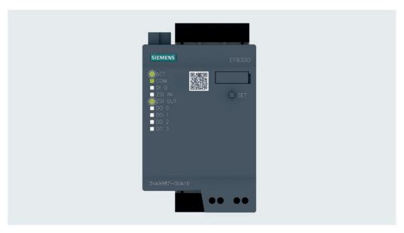
3. In order to activate the selected output, press the <SET> button for longer than 2 seconds.
