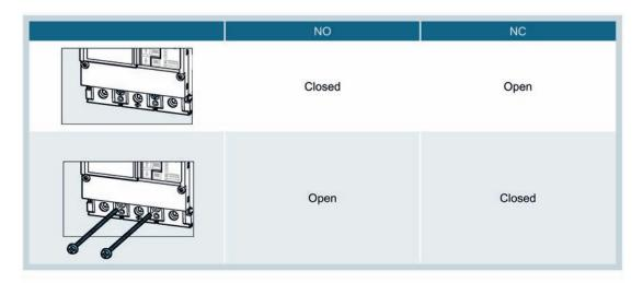
With this application, the position signaling switches indicate whether the molded case circuit breaker is inserted in the plug-in socket and secured by at least one screw. The reason for this application is that the molded case circuit breaker needs to be secured in position by mounting screws in the plug-in socket. All four mounting screws of the complete kit for draw-out technology must be used for this purpose.
