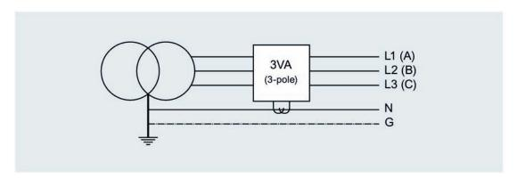
Trip unit variants, 3-pole 3VA6 molded case circuit breaker with external N transformer:
