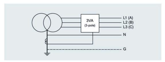
Trip unit variants, 3-pole 3VA6 molded case circuit breaker with external N transformer:
