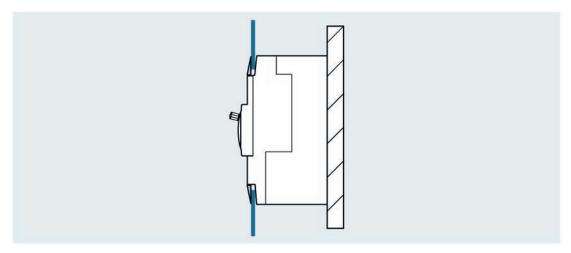
Handle and release are freely accessible, the panel door closes flush with the molded case circuit breaker.
