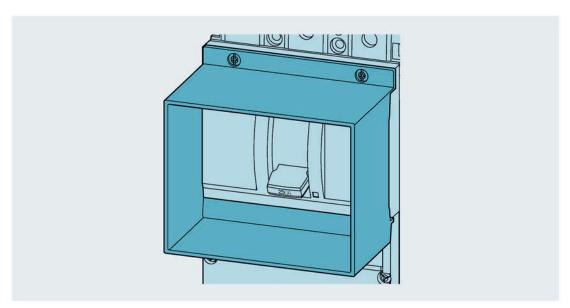
The door cutout must be positioned such that it is flush with the door feedthrough. It must also be positioned in such a way as to minimize the size of the gap between the feedthrough
