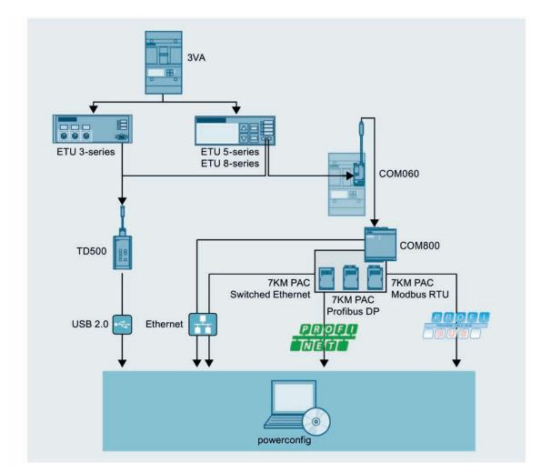
The possible means of connection of the COM800 / COM100 breaker data server are described in detail in the 3VA Communication system manual (see Reference documents (Page 11)).
