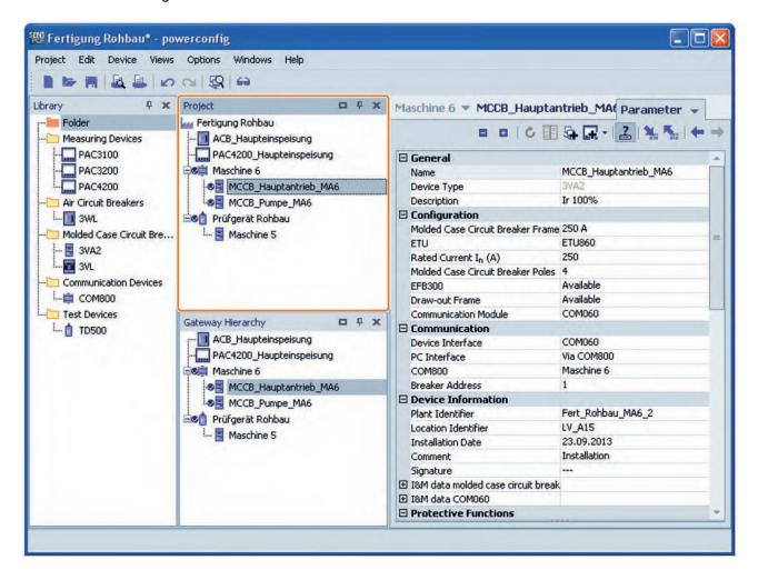
Electronic trip units (ETU), the EFB300 external function box and the communication structure can be commissioned easily by means of the powerconfig software. On completion of the commissioning process, the ETU settings can be stored as a project on the PC and printed out.
