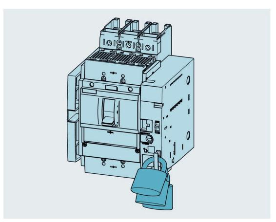
To provide protection against unauthorized operation of the molded case circuit breaker, padlocks can be inserted through the plastic frame opening of the padlock locking unit on the right side wall of the draw-out socket. The plastic frame is simple to pull out. The crank handle opening is mechanically sealed when the plastic frame is in the OUT position.
