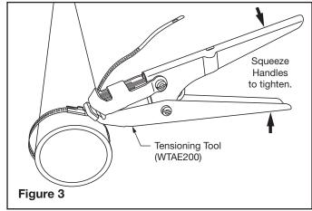
2. Tighten the Multi-Lok Cable Tie by either using the hand held tensioning tool, WTAE201 (Figure 2) or the tensioning tool, WTAE200 (Figure 3).
