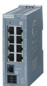
Preset for PROFINET mode! SCALANCE XB208 managed Layer 2 IE Switch 8x 10/100 Mbit/s RJ45 ports 1x console port; Diagnostics LEDs Redundant power supply temp. range 0 °C to +60 °C; mounting onto standard rail; Default PROFINET
