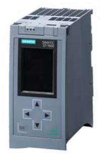
SIMATIC S7-1500, CPU 1516-3 PN/DP, Central processing unit with Work memory 1 MB for program and 5 MB for data, 1st interface: PROFINET IRT with 2-port switch, 2nd interface: PROFINET RT, 3rd interface: PROFIBUS, 10 ns bit performance, SIMATIC Memory Card required
