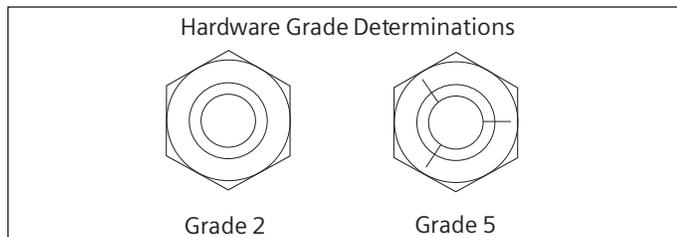
1) Older switchboards used Grade 2 hardware. See Hardware Grade Determination Detail for determining which type of bolt is installed in the gear. Also, refer to the torque table provided with the gear.
