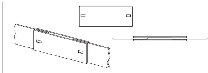
Figure 9 (Angle tie plate – Single hole)
