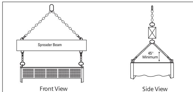
**3.4.2 Multi-section lifting** – The method of lifting a multisection unit is similar to lifting single section. The cables need to be connected to all lifting brackets. The lifting cables must have correct spreader from side to side (See Fig #1B). A crane with sufficient height and lift is required.
