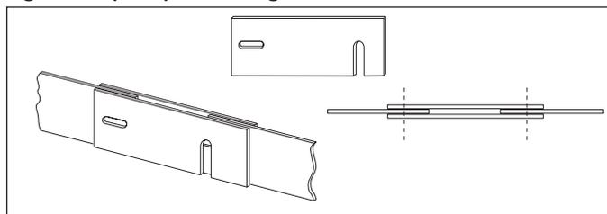
Figure 8 (Straight tie plate – Single hole)
