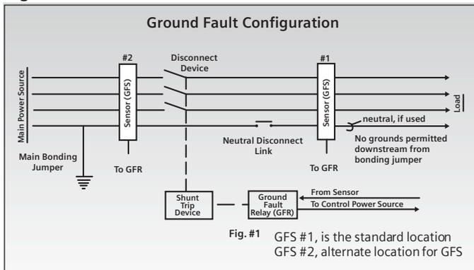
**WARNING:** The following should be performed only by qualified personnel as defined in NEC article 100. The ground fault sensor (GFS), ground fault relay (GFR), must be installed as in Figure 15.
