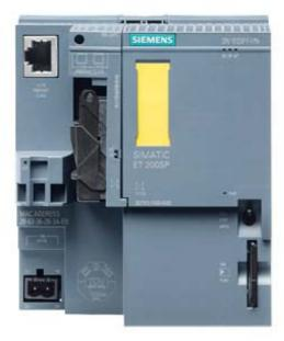
SIMATIC DP, CPU 1512SP F-1 PN for ET 200SP, Central processing unit with Work memory 300 KB for program and 1 MB for data, 1st interface: PROFINET IRT with 3-port switch, 48 ns bit performance, SIMATIC Memory Card required, BusAdapter required for Port 1 and 2
