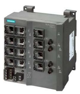
SCALANCE X112-2, Unmanaged IE switch, 12x 10/100 Mbit/s RJ45 ports, 2x 100 Mbit/s Multimode BFOC, LED diagnostics, errorsignaling contact with set button, redundant Power supply Manual available as a download
