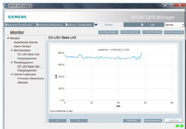
Trend diagram for load current in SITOP UPS Manager
