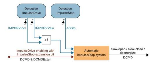
Figure 3-6 Automatic ImpulseStop system
