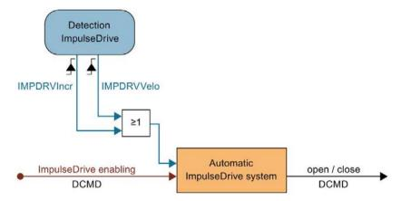
Figure 3-5 Automatic ImpulseDrive system
