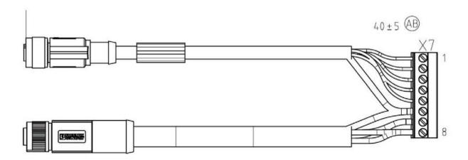
Figure 5-12 Motor cable MDG2 CABLE
