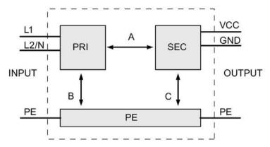
Figure 6-7 Diagram test voltage
