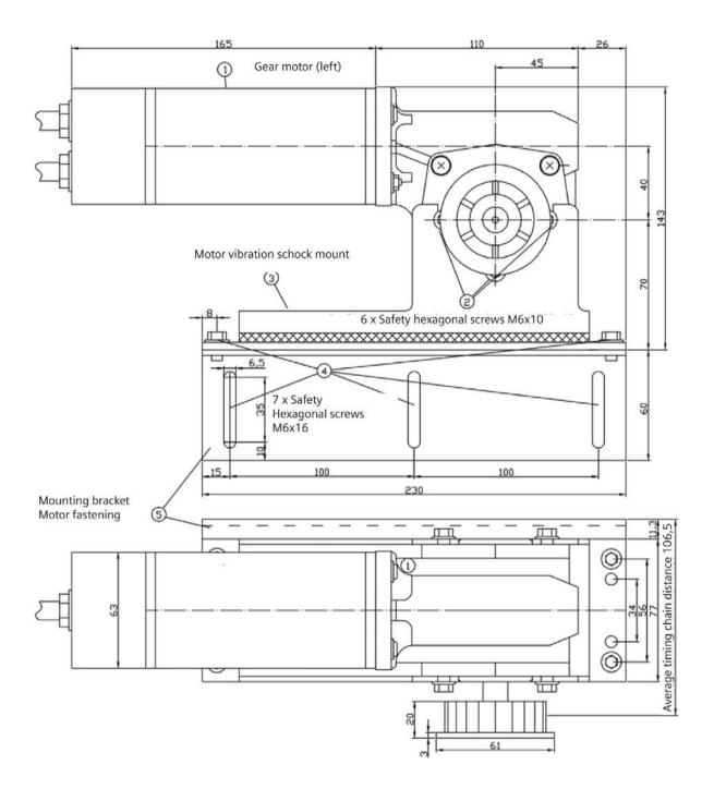
Figure 5-6 Geared motor with rubber-metal anti-vibration mount and mounting bracket (M4 motor)
