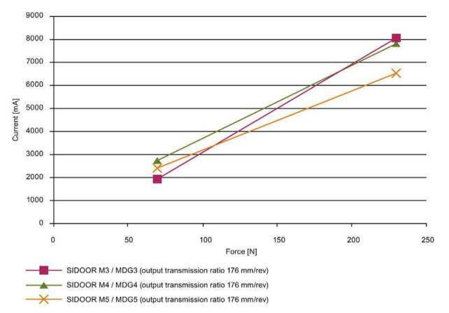
Figure 4-11 Current – force – motor characteristic in closing direction for output transmission ratio 176 mm/rev
