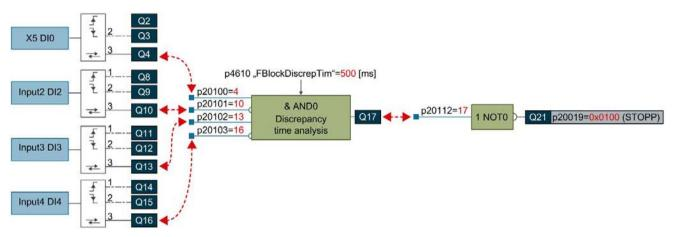
Figure 3-16 Two-hand control device example parameterization
