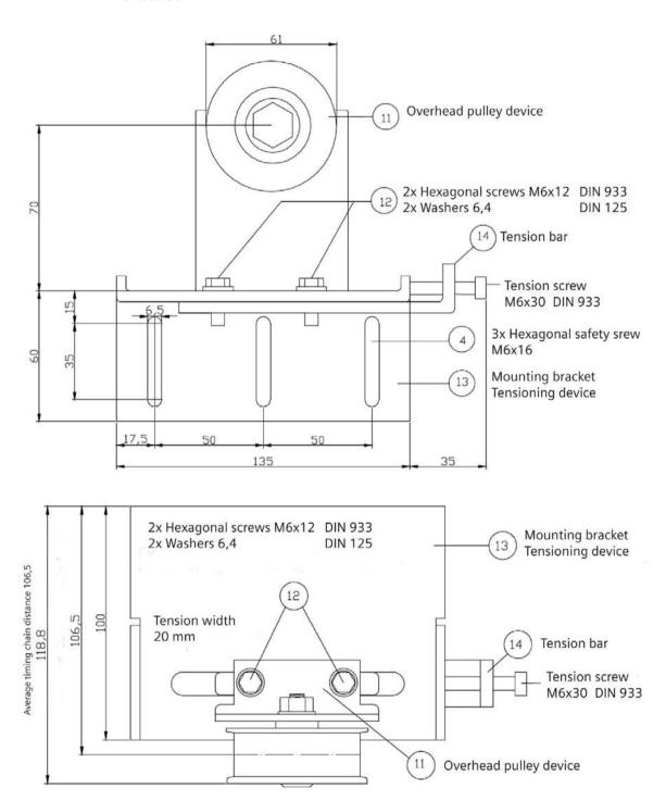
Figure 5-13 Deflector pulley with tensioning device and mounting bracket
