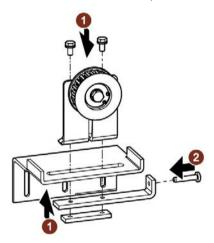
Ensure that the drive pinion and deflector pulley are aligned when doing so. They have to be exactly aligned to ensure a long drive service life.
