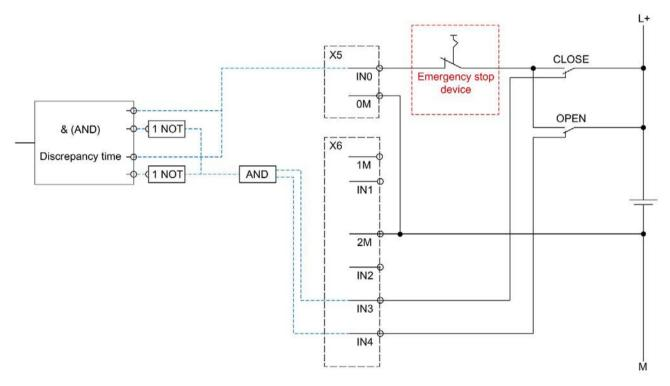
Figure 3-21 Interfacing safe (PLd) digital door control (OPEN/CLOSE) with emergency stop (encoder type 1) via 3 digital inputs
