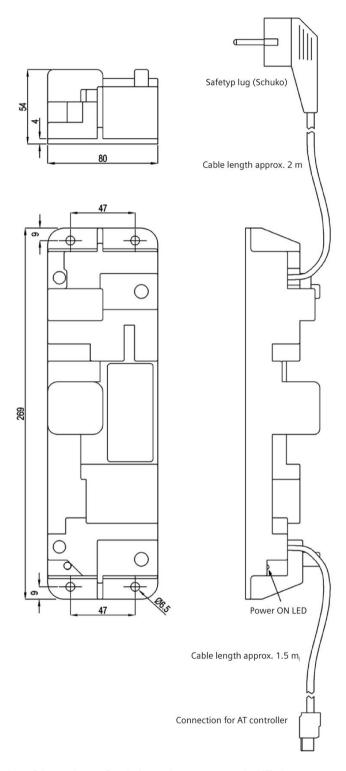
Figure 6-2 Dimensions of switch mode power supply NT40
