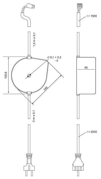
Figure 6-5 Dimensions of the SIDOOR TRANSFORMER
