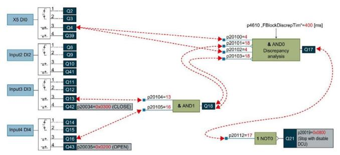
Figure 3-22 Example emergency stop parameterization (digital control) via 3 digital inputs
