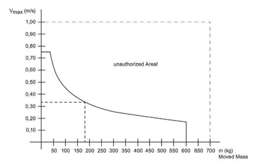
Figure 3-3 Speed limit curve for W<sub>KIN</sub>=10Y
