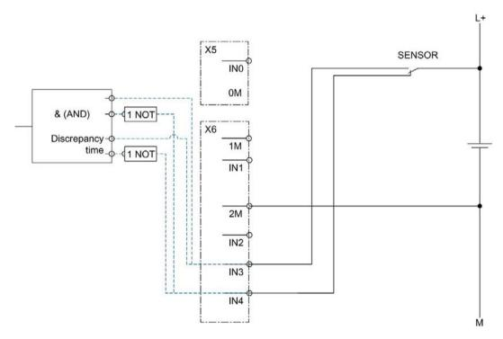
Figure 3-12 Connect the switchgear to the change-over contact, 2-channel nonequivalent
