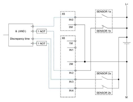
Figure 3-15 Two-hand control device example
