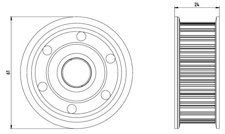
Figure 5-15 SIDOOR MDG Pulley transmission ratio 176 mm/rev
