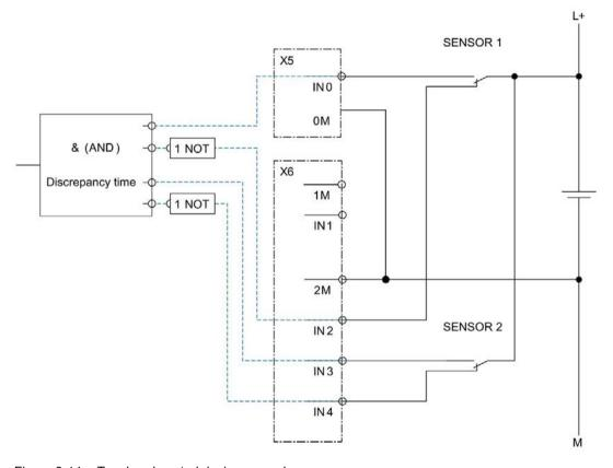
Figure 3-14 Two-hand control device example
