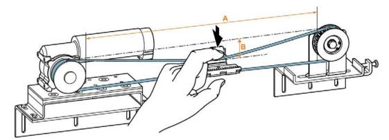
You will recognize the correct belt tension by how far the belt is pressed in (B). The depth (B) the belt is pressed in depends on the distance between the drive pinion and deflector pulley (A).
