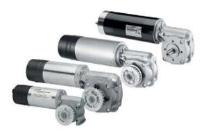
Geared motors form the maintenance-free drive unit in the door drive. The geared motors feature DC motors with non-self-locking gearing and are speed-controlled. The set force and speed limits are not exceeded.
