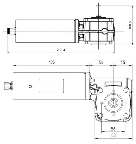
Figure 5-8 Dimension drawing SIDOOR MDG4
