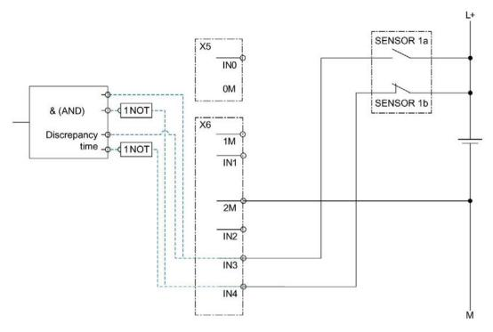
Figure 3-13 Connect the switchgear to two separate non-equivalent change-over contacts, 2-channel non-equivalent\*
