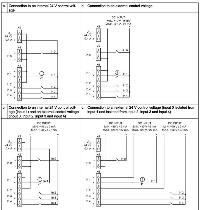
① Light barrier, DCPS sensor, jumpered or switch. The wiring depends on the sensor type and the configuration of Input 1.
