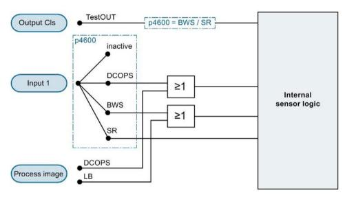
Figure 4-5 Sensor signals
