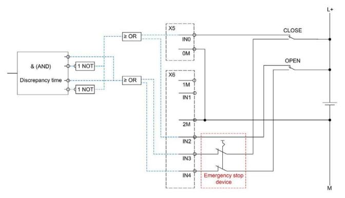
Figure 3-18 Interfacing safe (PLd) digital door control (OPEN/CLOSE) with emergency stop (encoder type 1) via 4 digital inputs
