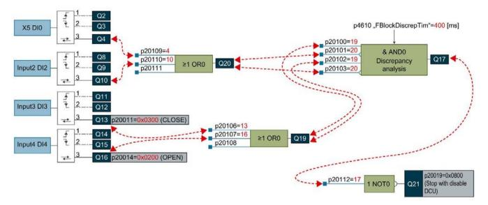
Figure 3-20 Example emergency stop parameterization (digital control) via 4 digital inputs
