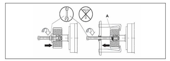
Figure 5-2 Fitting and removing output elements; A = intermediate washer (for maintaining the centering in the shaft extension)
