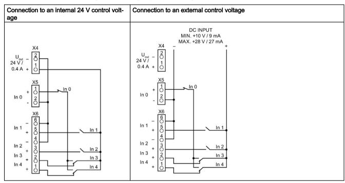
Table 4-4 Terminal circuit diagrams for emergency stop with 3 digital inputs
