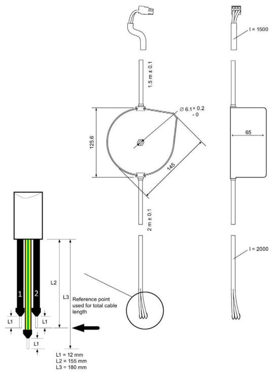
Figure 6-8 Dimension drawing TRANSFORMER UL
