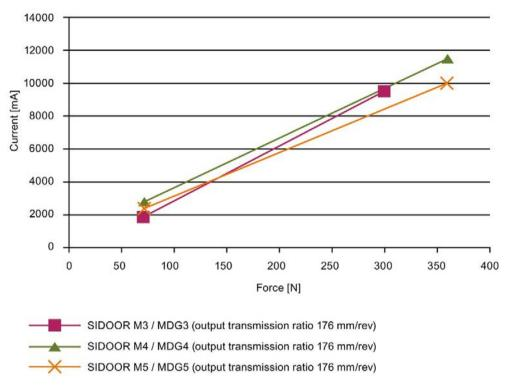
Figure 4-10 Current – force – motor characteristic in opening direction for drive transmission ratio 176 mm/rev
