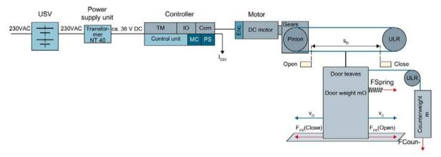
Figure 6-10 SIDOOR system block diagram
