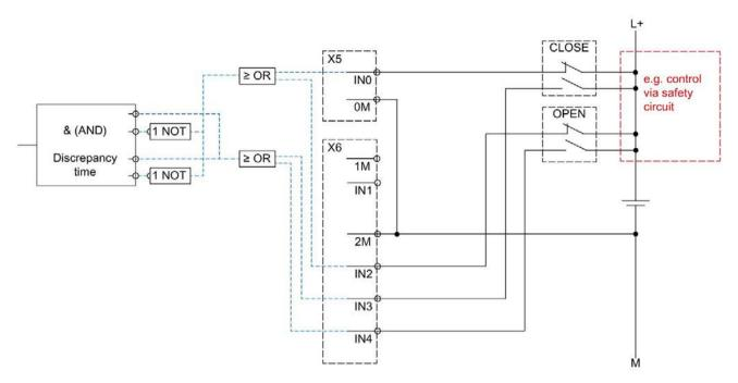
Figure 3-19 Interfacing safe (PLd) digital door control (OPEN/CLOSE) with emergency stop (encoder type 2)
