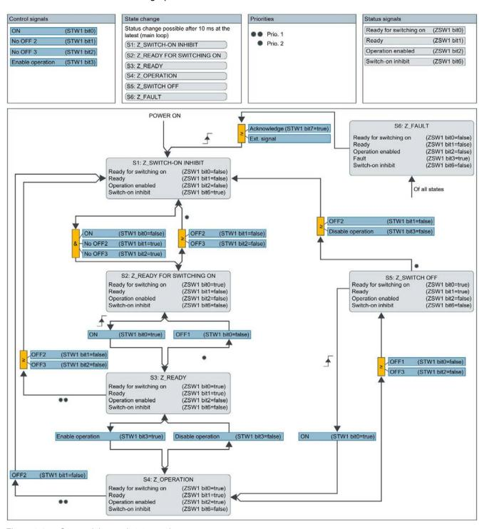
Figure 4-4 Sequential control state graph
