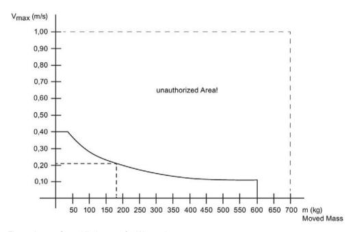
Figure 3-4 Speed limit curve for W<sub>KIN</sub>=4J
