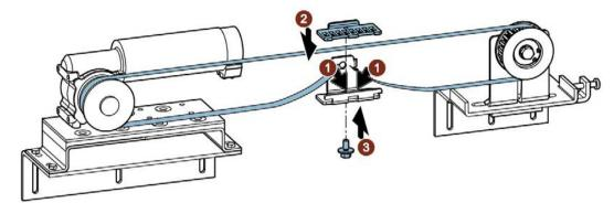
4. Tension the toothed belt with the aid of the tensioning device.
