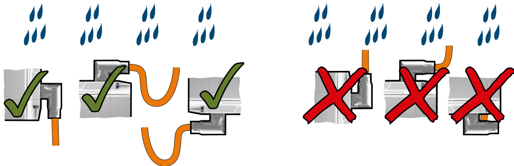
Figure 5-7 Permissible and impermissible cable routing when connecting in a damp environment
