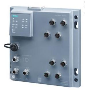
SCALANCE XP208, managed IE switch, 8x 10/100 Mbps M12 ports, IP65, LED diagnostics, error signaling contact, Redundant power supply, PROFINET IO device, network management, operable in redundant ring, Dust caps, incl. electronic Manual on CD-ROM, Cplug optional
