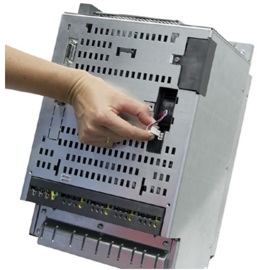
4. Withdraw the connector. To do so, gently press the interlock and connector together.
