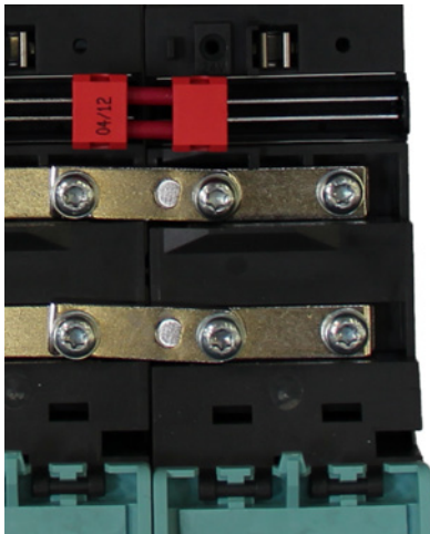
Figure 8-4 Motor Modules with 24 V connector installed
