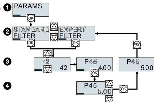
3. Select the required number of a write parameter using the arrow keys.
