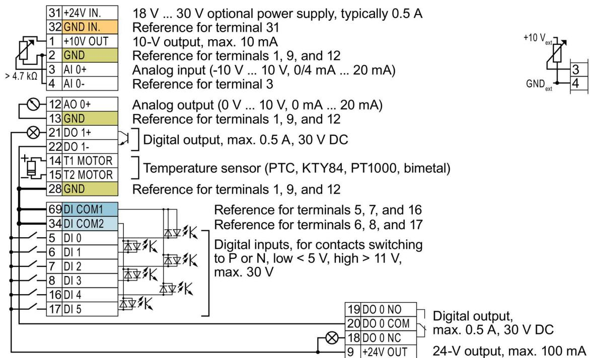
**GND** All terminals with the reference potential "GND" are connected to each other inside the inverter.
