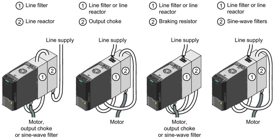
Image 3-5 Permissible combination of two base components
