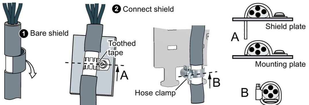
Image 3-8 EMC-compliant shield connection
