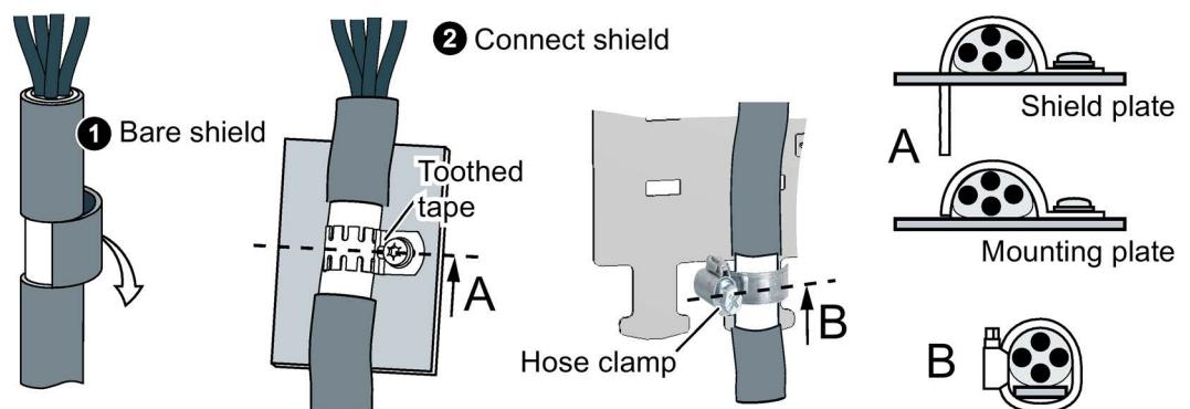
Image 3-8 EMC-compliant shield connection
