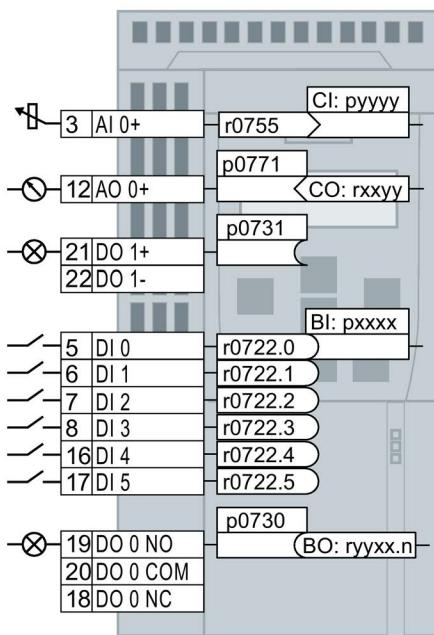
The function of the terminal is defined through a signal interconnection in the inverter:
