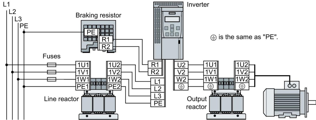
Image 3-6 Connecting the inverter and its optional components
