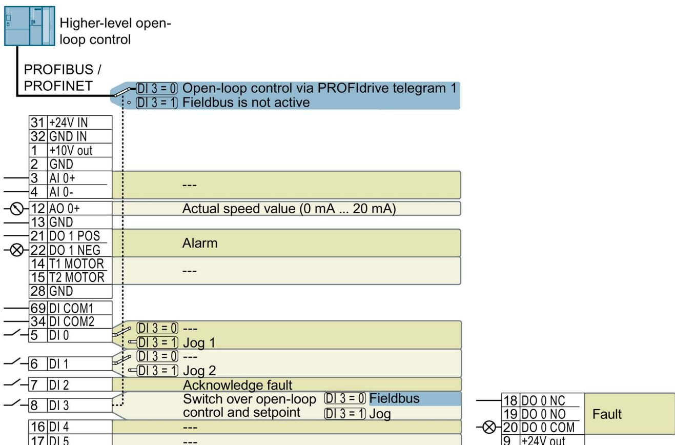
Image 3-11 Factory setting of the terminals for G120C DP and G120C PN
