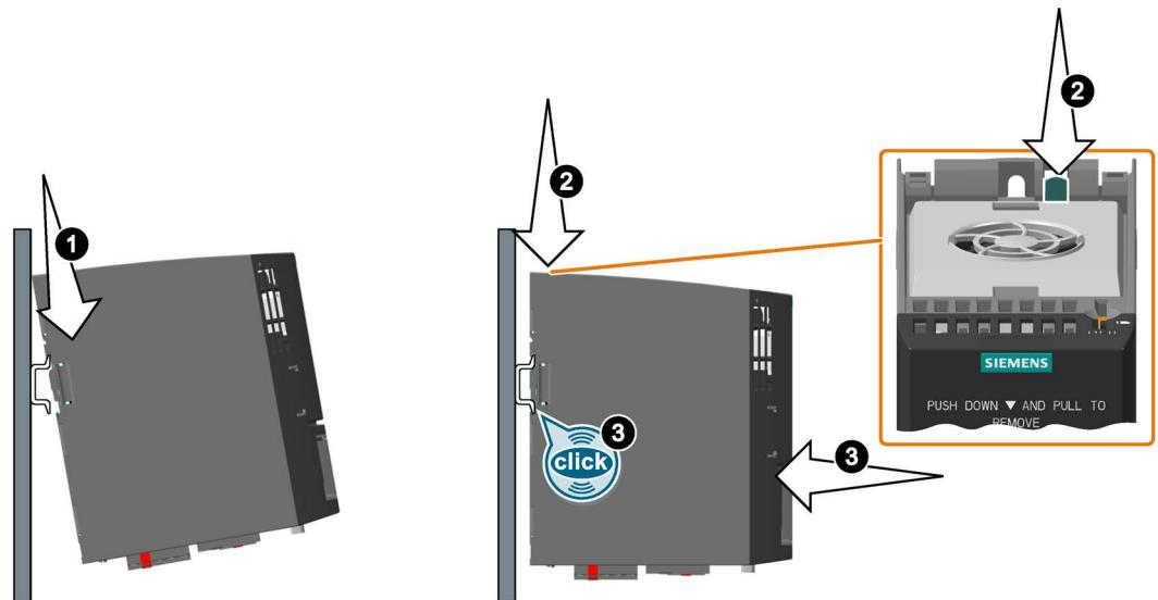
Image 3-3 Mounting on a standard mounting rail
