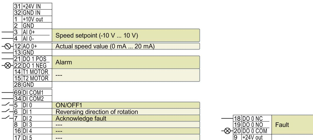
Image 3-10 Factory setting of the terminals for G120C USS and G120C CAN
