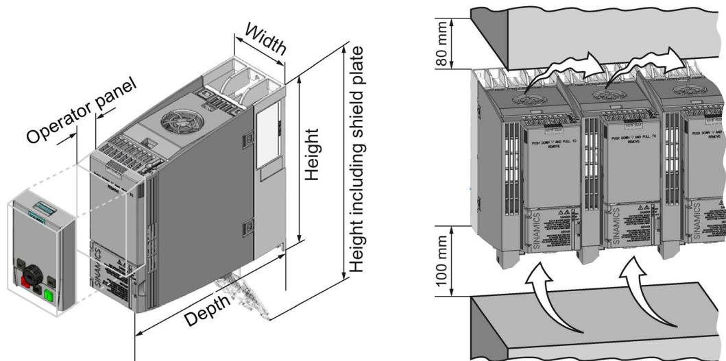
Image 3-1 Dimensions and minimum spacing to other devices
