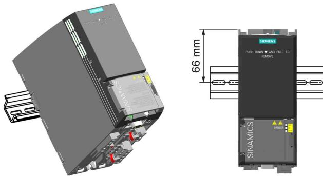
You can mount inverters, frame size FSAA on a TS 35 mounting rail.
