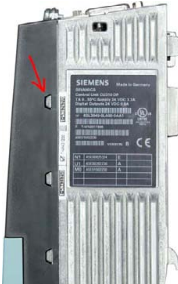
Figure 11-1 Lateral snap hooks on a CU310 DP
