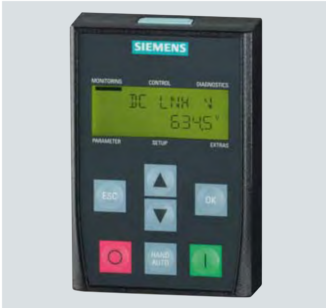
Basic Operator Panel BOP-2
