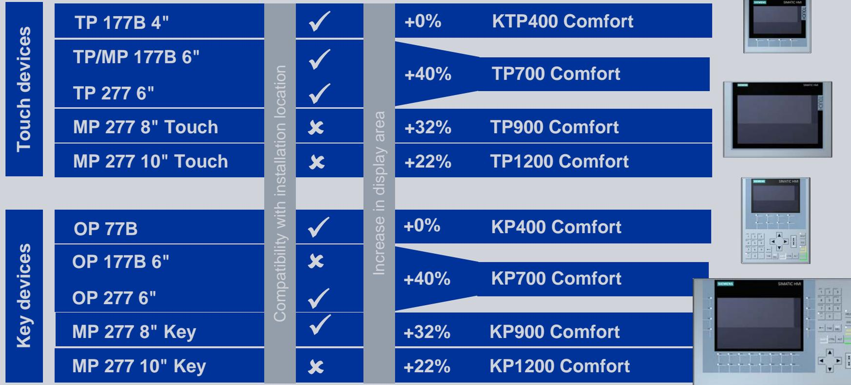
The widescreen displays increase usable display area by up to 40 percent when compatible with the installation location.
