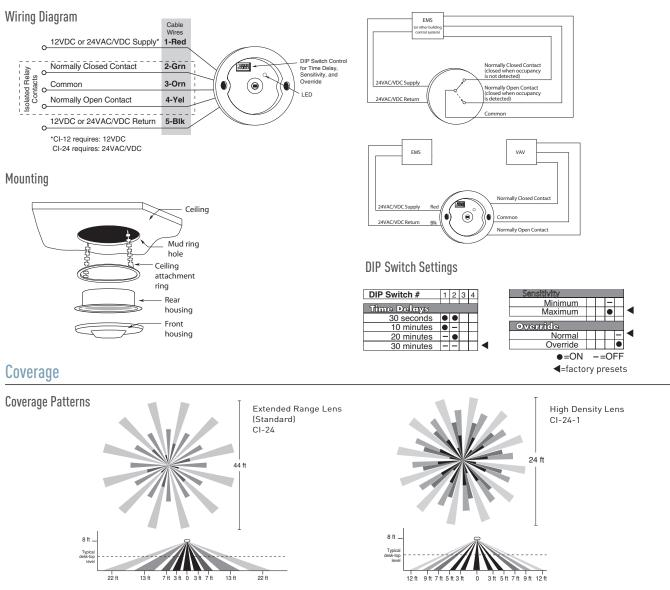
Coverage shown is maximum and represents coverage for half-step walking motion. Under ideal conditions, with no barriers or obstacles, coverage for half-step walking motion can reach up to 1200 ft<sup>2</sup> using the Extended Range lens and up to 500 ft<sup>2</sup> using the High Density lens. For typical desktop level of activity, coverage can reach up to 300 ft<sup>2</sup> using the High Density lens.
